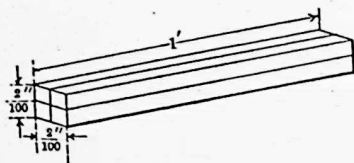
FIG. 82. One wire 2 in. square makes four wires 1 in. square.
