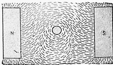
FIG. 137. The shape of the magnetic field is due to the current in the wire and the field between the two poles.
