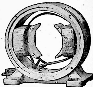
FIG. 115. Westinghouse two-pole motor or generator.
